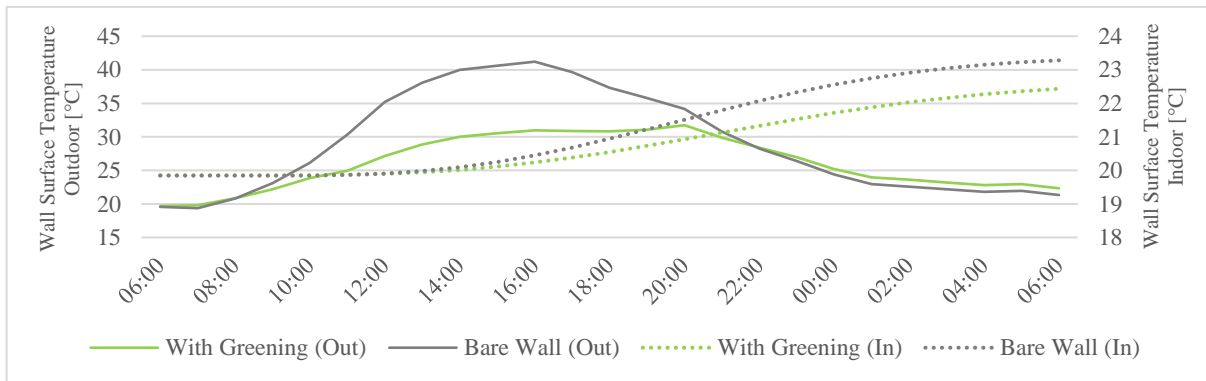
Fig. 3: Wall surface temperatures with and without greening (Madrid, LAI=1, 2 nd floor, south façade)
