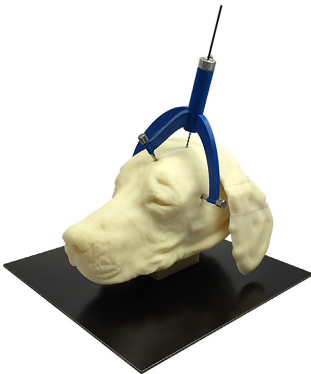
FIGURE 1 A dog model with a personalized, 3D printed stereotactic brain biopsy device connected to the head via bone anchors and screws with the biopsy needle in place
