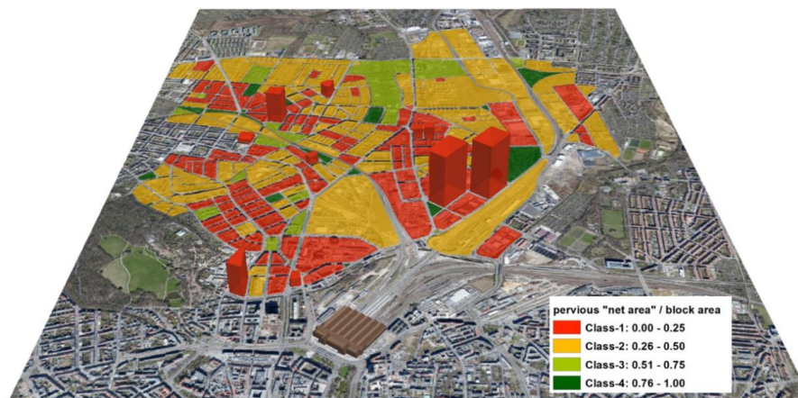
Figure 7. Simulation result of scenario 4, depicting the trough-trench infiltration for a 30-year rainfall event on a soil with high permeability ( k_f = 10^{-4} m/s). The columns represent the amount of runoff from the blocks and are not true to scale for presentation purpose.
