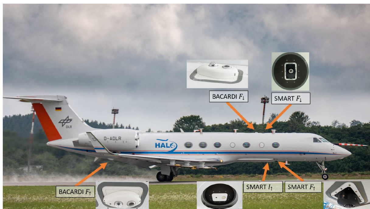
Figure 2: HALO during landing with the locations of the different radiation sensors. Photo: Andreas Minikin; Instrument photos: Roger Riedel, Hanno Müller.
