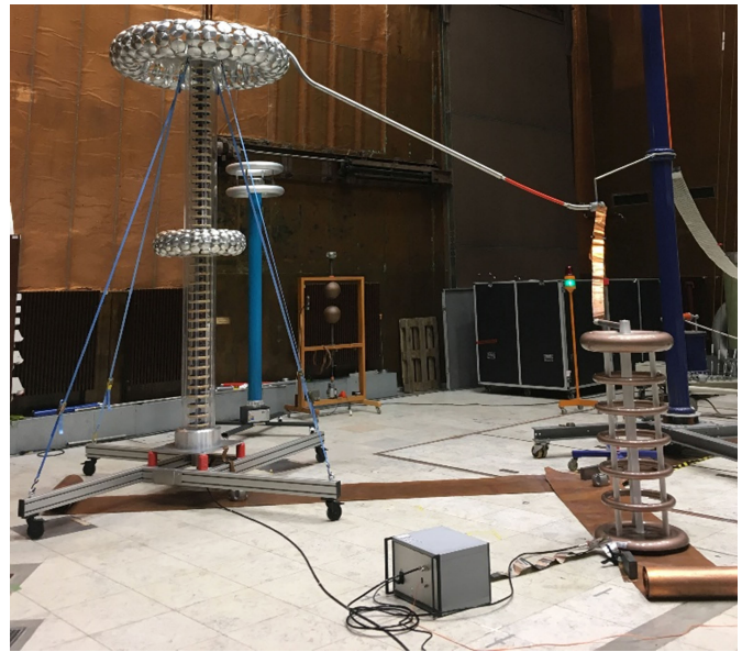
Fig. 5. Measurement arrangement for the high-voltage impulse tests. The system under test (VTT) with its digitizer is on the right side of the photograph. The voltage divider of the other system (PTB) to measure the stability of the generator is on the left side of the photograph.
