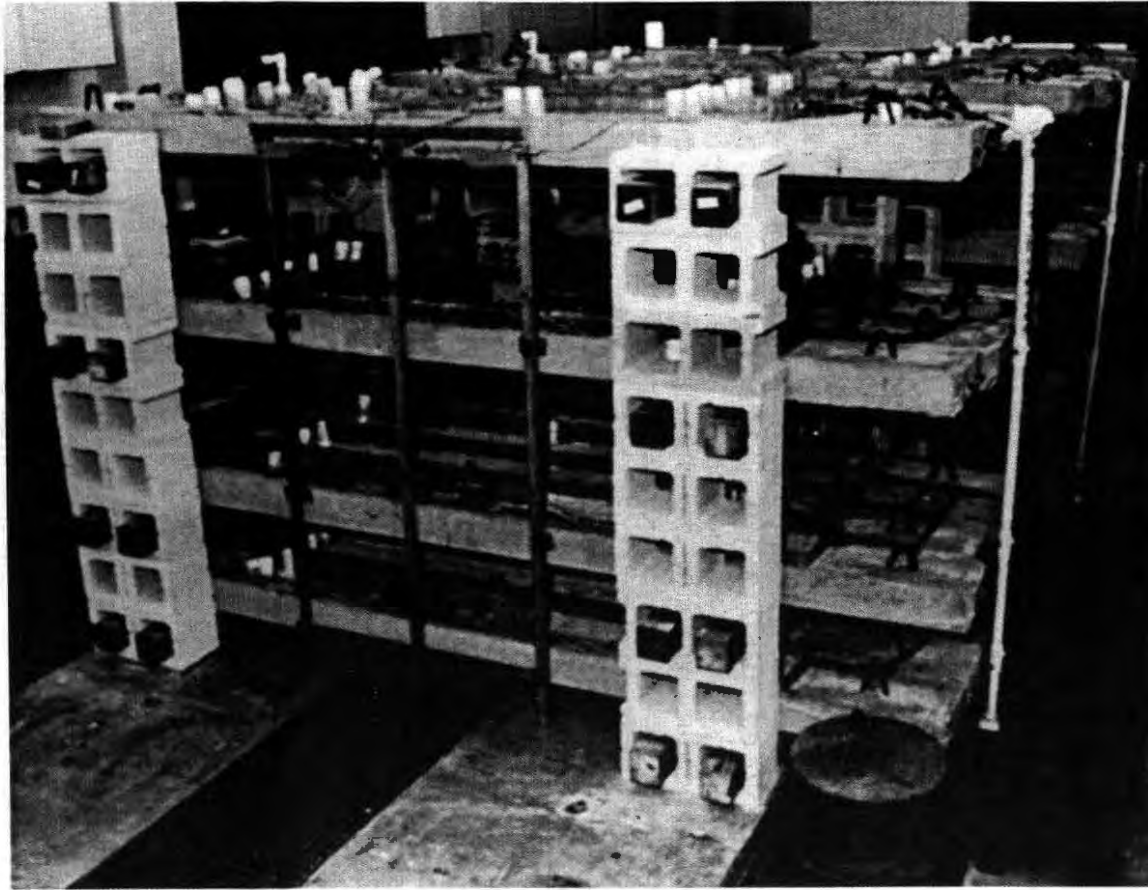
Figure 9: Photograph of prestressed concrete beam in position in the laboratory.
