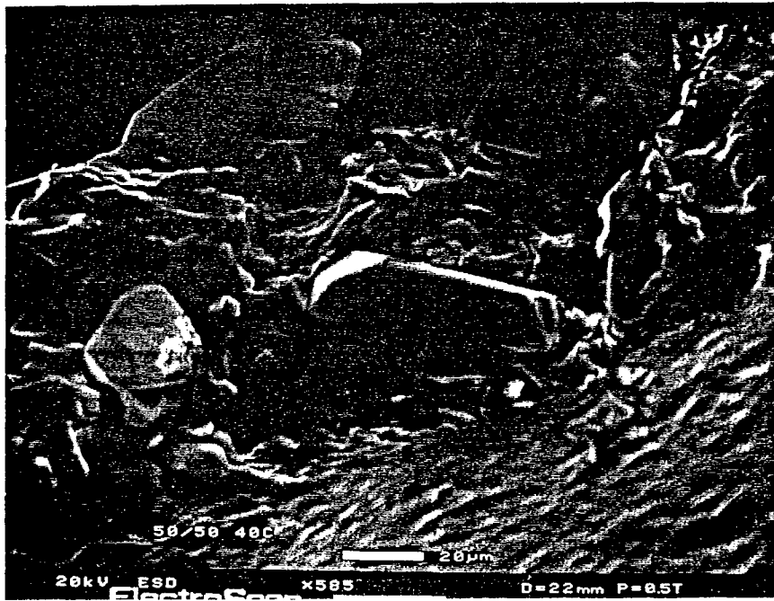
Figure 18. Scanning Electron Micrographs of the 50/50 (198:233) two-pot blend binder from (a) the surface, and (b) the interior at 40 °C (104) using the ESEM.
