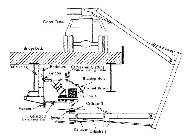
Figure 2. Overall view of the RBPR system design.
