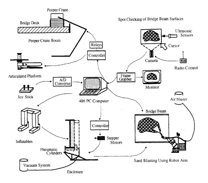
Figure 5. Modularized control system architecture for the RBPR.
