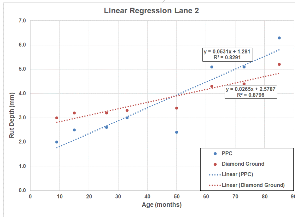
Figure 10. Lane 2 wear measurements for the PPC and Diamond Ground sections. Wear rate per year is equal to 12 times the slope of the line.
