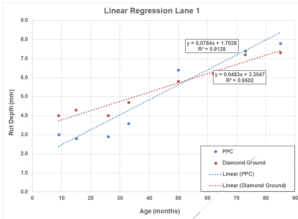
Figure 9. Lane 1 wear measurements for the PPC and Diamond Ground sections. Wear rate per year is equal to 12 times the slope of the line.
