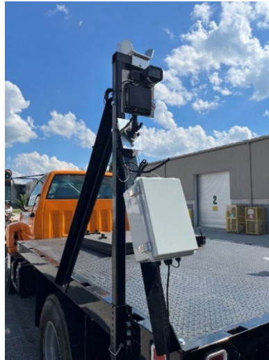
Figure 12. TMA install for Move Over Law system.
