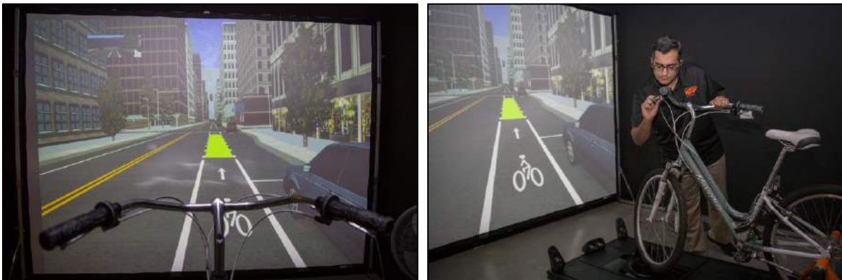
Figure 0.2 Simulated environment in the OSU Bicycle Simulator. Left: Participant's perspective. Right: Outside view, with researcher checking the bicycle brake
