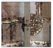
The disk-shaped compact tension test is a standard way to understand the crack resistance of asphalt.
