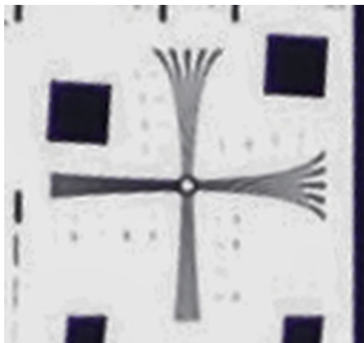
Figure 54. Closeup of Figure 53 Showing the Resolution Limit at 3 mm
