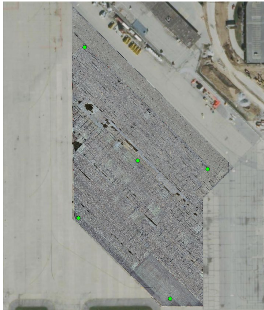
Figure 71. Five GCP Locations Over the Remote Aircraft Parking Apron 1 South at CVG
