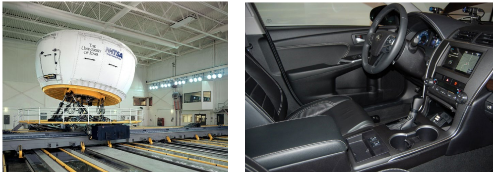
Figure 2. Exterior and interior views of the NADS-1 simulator
