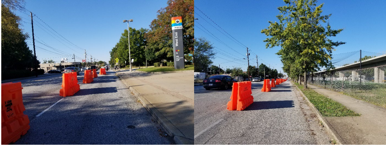
Figure 13. Temporary multiuse lanes on Lee Street SW, Atlanta, GA. Image Credit: Temporary multiuse lanes by Atlanta Department of Transportation. Permission to use granted by ATLDOT.
