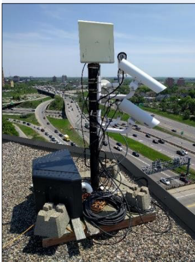
Rooftop video cameras captured real-time vehicle data used to assess traffic conditions.
