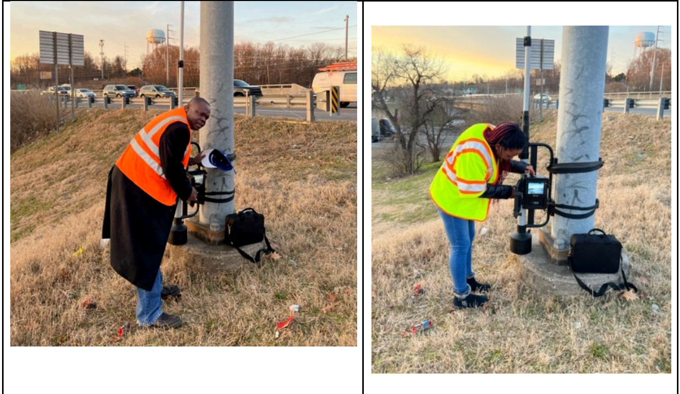
Figure 4.6: Traffic data collection using Miovision Equipment
