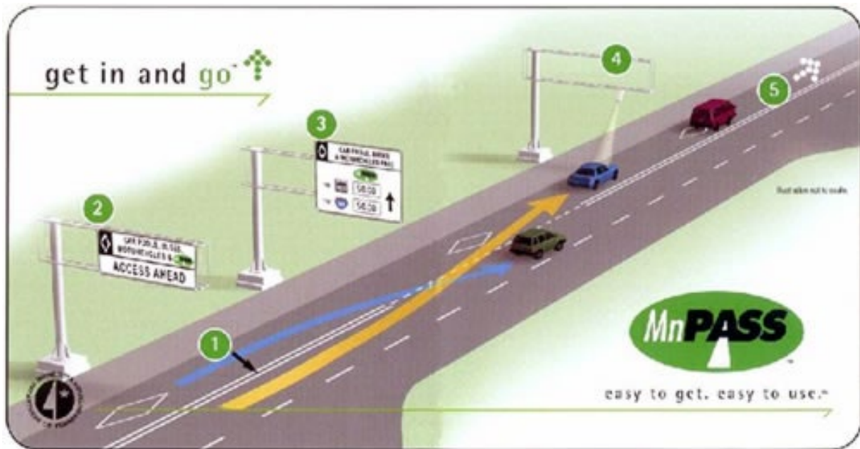
Figure 2.3: HOT Lane Access Road Geometry in Minnesota
