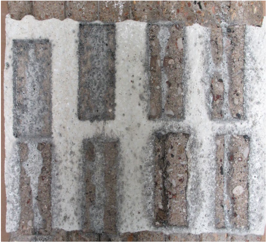
Figure 5: Photograph of a white hot tape stripe on concrete specimen with different ablated regions.
