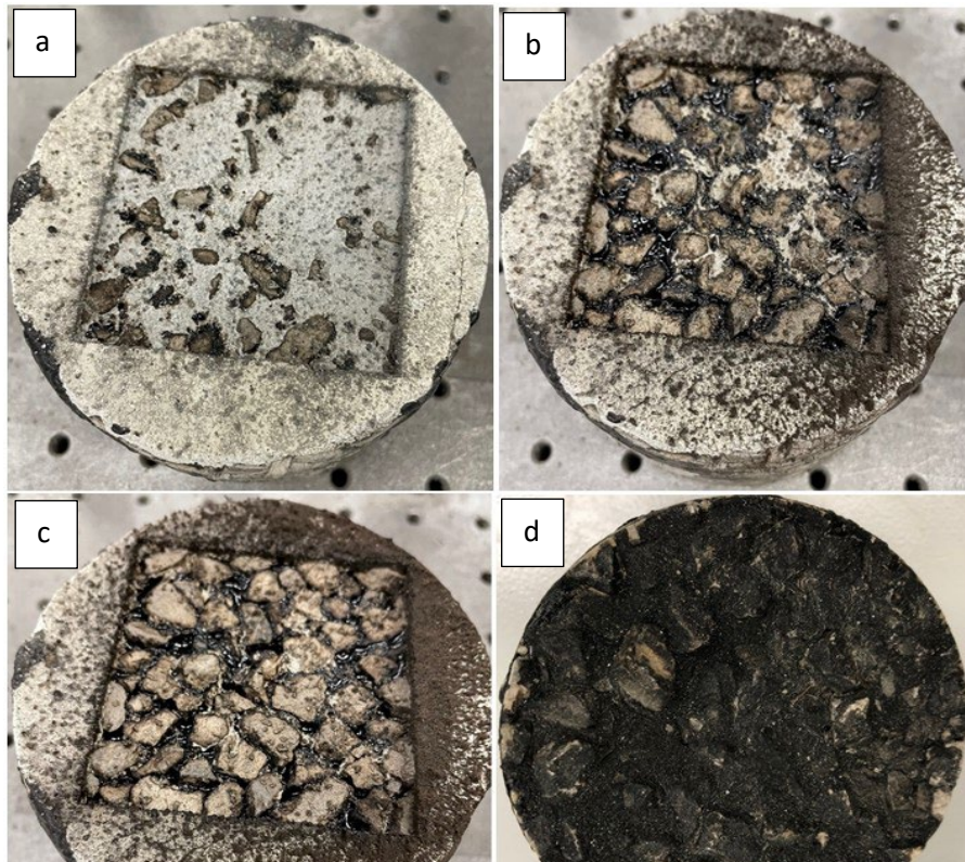
Figure 7: Removal of paint stripe from asphalt by multiple scans: a) first scan; b) second scan; c) third scan; d) control.
