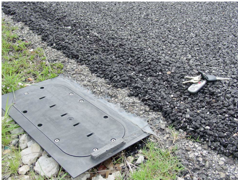
Figure 8. Photograph of Installed Sampler at Edge of Pavement (26)
