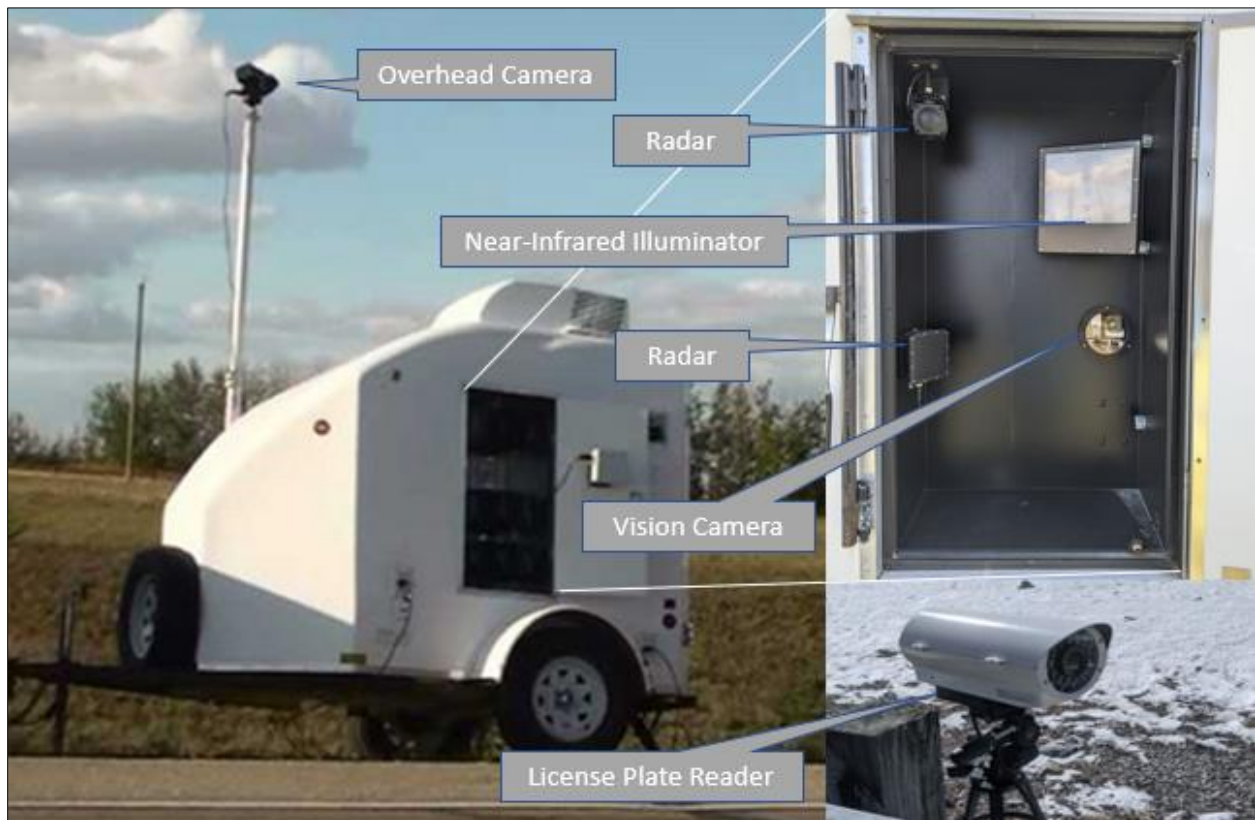
Figure 1. Mobile Automated Placard Reader System (APRS) Trailer with System Component Types and Locations Shown
