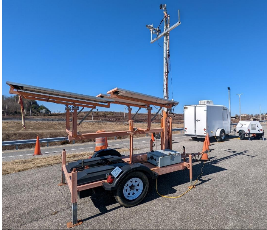
Figure 4. View of the Sensor Trailer with the Mobile APRS and Generator Shown in the Background
