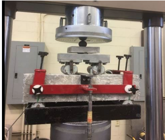
Figure 5.34 Test setup for flexural strength
