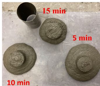
Figure 3.1 Undisturbed and disturbed slump spread test
