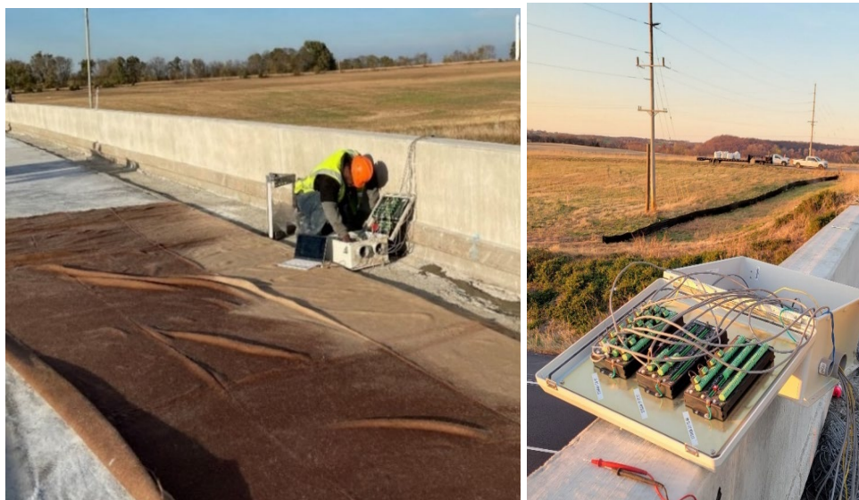
Figure 5.36 Connection to DAQ box for Route Z Bridge (left) and Route M Bridge (right)
