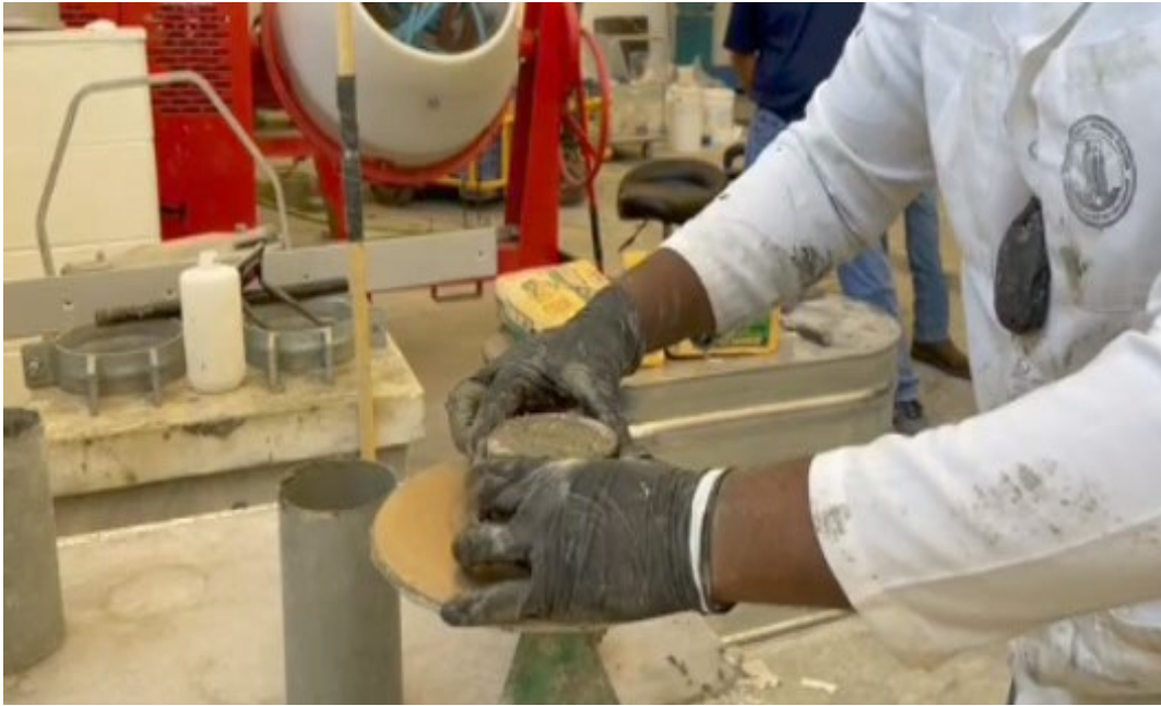
Figure 5.3 Slump flow test
