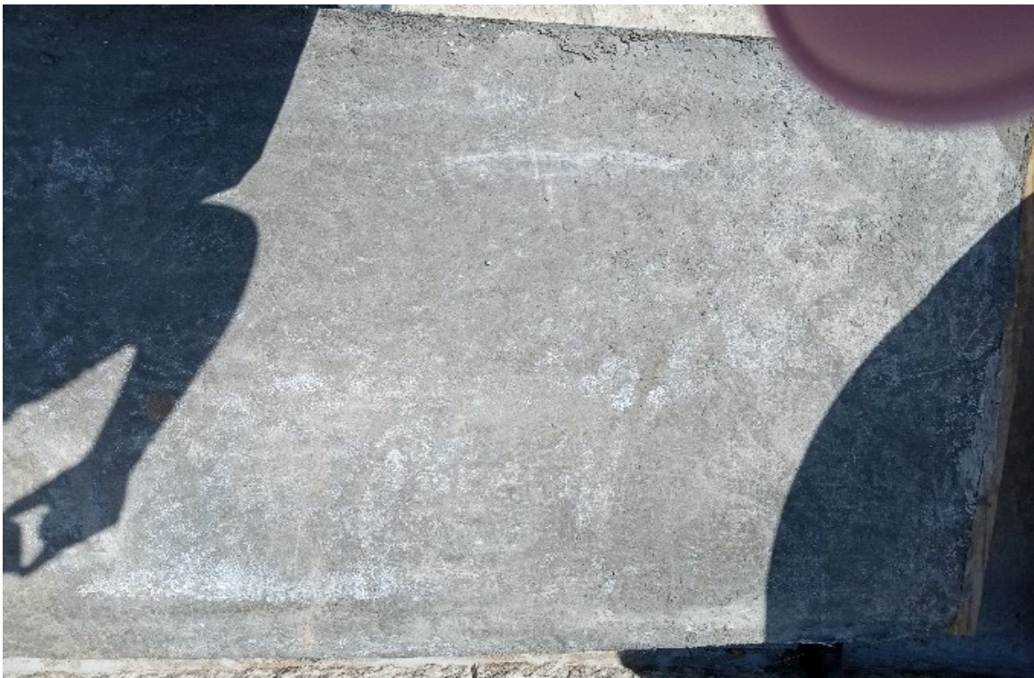
Figure 5.6 Surface of mockup overlay after approximately 8 months of outdoor exposure showing intact surface with no surface cracking
