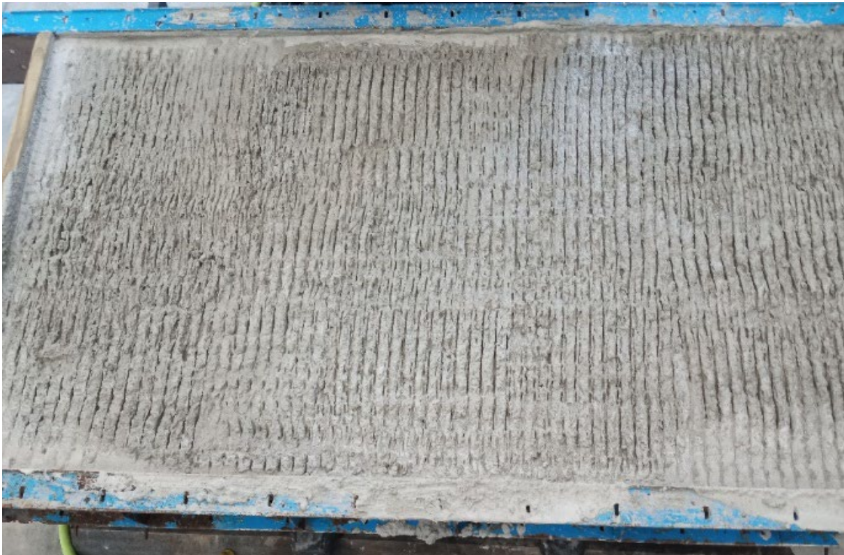
Figure 5.1 Concrete substrate surface prepared using scarification and water blasting
