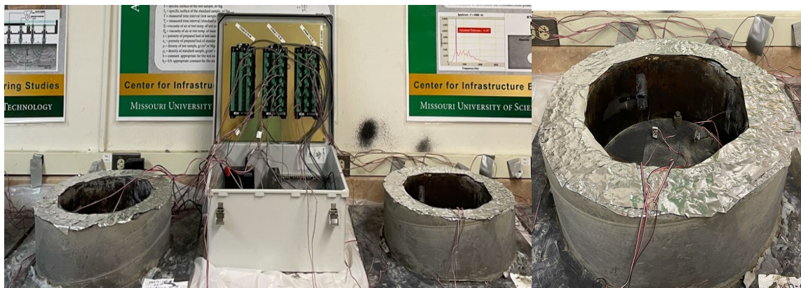
Figure 3.4 Restrained shrinkage test
