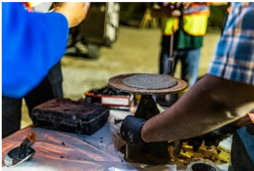
Figure 5.9 Slump flow testing of UHPC used in field mockup
