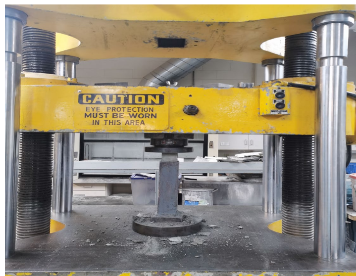
Figure 5.33 Compressive strength test
