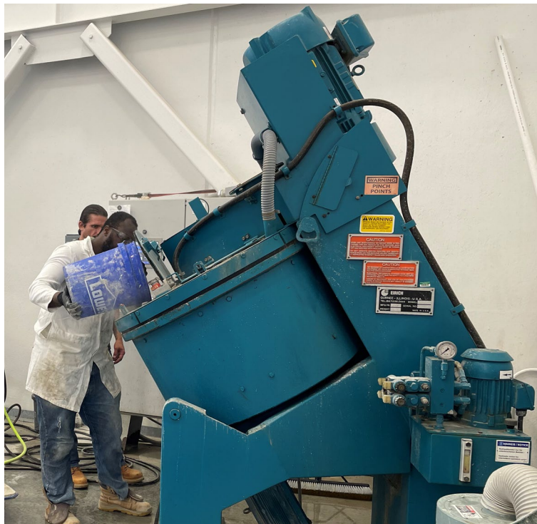
Figure 5.2 High-shear EIRICH mixer
