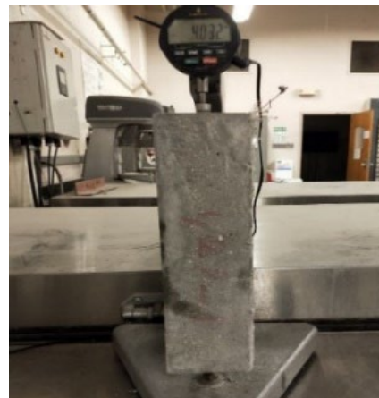
Figure 5.35 Digital-type extensometer for drying shrinkage
