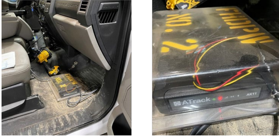
Figure 14. SkyHawk Portable AVL Equipment for Street Sweeper Vehicles
