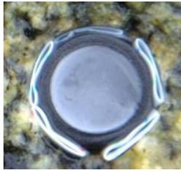
field trips using liquid wax introduced in small round plastic containers of around 1 cm of diameter. In the field, a drill with the similar height and diameter of the tablet was used to create a hole where the tablet was fixed. To prevent its loss by wave exposure, small pieces of straw were placed around the space left between the rock and the tablet (Figure 12).
