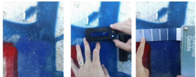
Fig. 17. Comparative study of the data obtained with the sensor and the color chart (graffiti 1) (Redmi Note 8 Pro, Xiaomi f/1.89, 1/168, ISO100, 5.43mm, without Flash) (Redmi Note 8 Pro, Xiaomi f/1.89, 1/162, ISO100, 5.43mm, without Flash).
