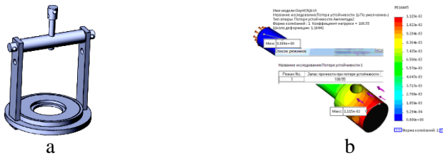
Figure 5 – Geometric a model of the bearing puller (a) and resulting amplitude and safety margin with loss of stability (b)
