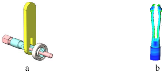
Figure 6 – Screw puller of bearings from crankshaft (a) and epura distribution of total stresses von Mises tsanga (b)
