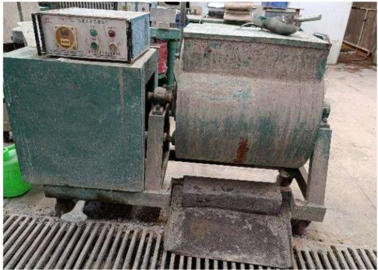
Figure 5-6. The concrete horizontal mixer
