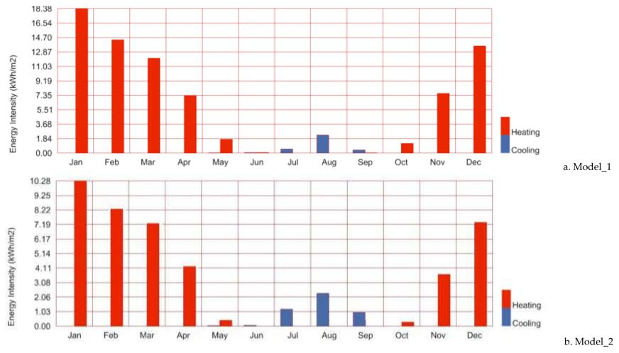
Figure 6-13. The energy comparison before and after renovation (a. Model\_1 b.Model\_2)
