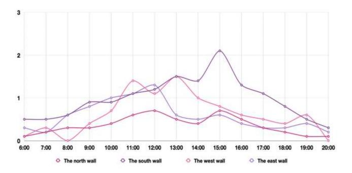
Figure 4-23. The temperature variation of inner walls in Case A
