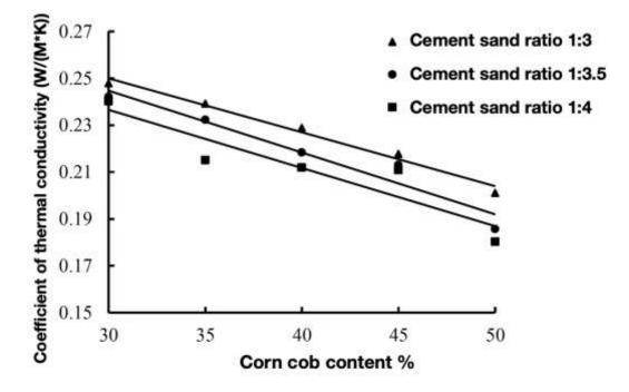
Figure 5-10. The thermal conductivity curve to the corncob volume content
