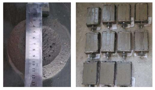
(b) Measurement of fluidity of reclaimed mortar (c) Molding of reclaimed mortar Figure 5-5. The test situation of reclaimed mortar
