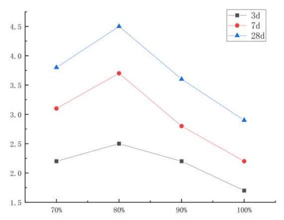
Figure 5-9. The compressive strength of concrete under different water consumption of corncob
