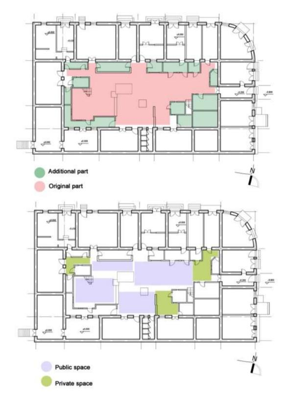
Figure 4-10. The spatial arrangement in the central atrium including private extension and isolation of toilet
