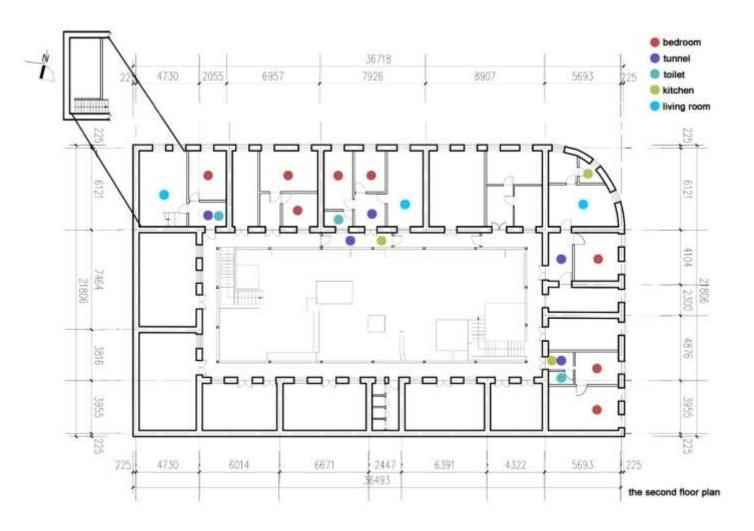
Figure 4-11. The detailed layout of the 2nd floor in Case A
