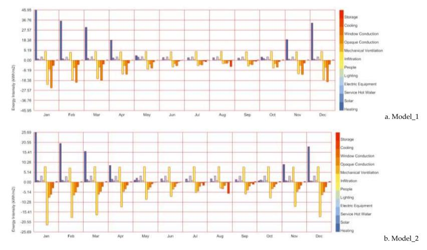
Figure 6-14. The energy balance before and after repair (a.Model\_1 b.Model\_2)
