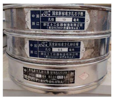
Figure 5-3. The standard square hole sieve
