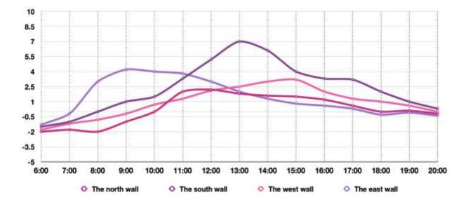
Figure 4-22. The temperature variation of outer walls in Case A
