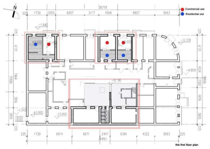
Figure 4-9. The analysis of the detailed layout on the first floor of Case A
