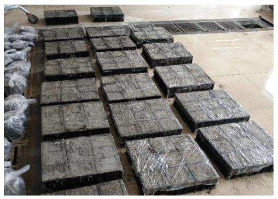
Figure 5-7. The concrete with formwork maintenance
