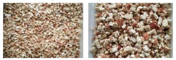
(a)4.75mm-9mm (b) 9mm-19mm Figure 5-4. The corncob particles with different particle size ranges
