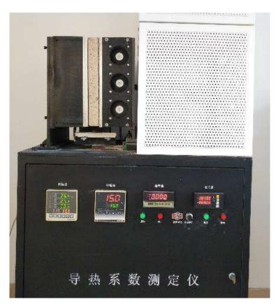
Figure 3-3. The appearance thermal conductivity tester
