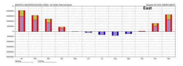
Figure 6-26. The monthly heating and cooling when change EAST facade Table 6-22. The data of monthly heating and cooling loads when changes EAST façade
