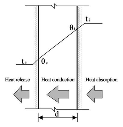
Figure 3-4: The experimental schematic diagram of heat transfer coefficient of materials
