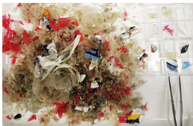
Figure 3. An example of separated CMP fraction according to the polymeric components.
