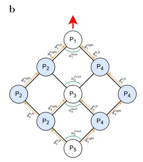
longitudinal deformation tests, respectively. White and blue colours indicate modules with a symmetric and asymmetric neighbourhood, respectively. The red arrow indicates the Kilobot Soft Robot's forward direction.
