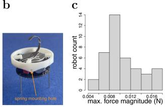
thereby constraining the movements (and orientation) of the module. c Maximum magnitude of force a module can exert onto a single spring (based on 40 robots, each subjected to five independent trials).
