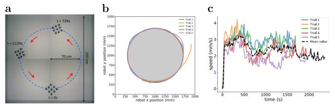
Fig. 3 | Physical experiment in which 3 × 3 Kilobot Soft Robots are programmed to follow a reference trajectory with closed-loop control. a Bird's-eye view of the experimental area, generated by superimposing snapshots taken from a typical experimental trial. The reference trajectory (dashed circle) is a circle of radius 70
