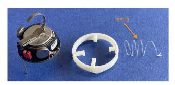
**Fig. 5** | **Overview of the module of the Kilobot Soft Robot.** a Up to four helical springs can be connected to the Kilobot through a 3-D printed circlet. **b** Kilobot equipped with the circlet. The circlet is firmly attached to the Kilobot (i.e. the latter can not rotate within the circlet). Four springs are attached at fixed mounting holes,
