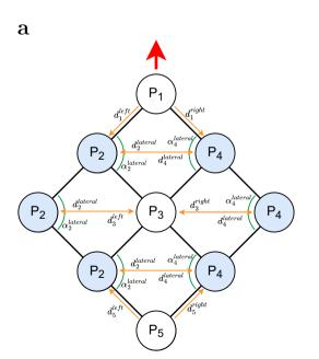
Fig. 6 | The modules of the Kilobot Soft Robot use their localisation estimates to identify any deviations from the reference shape (square lattice). a, b show the set of distances and angles considered by Algorithm S1 during the lateral and
