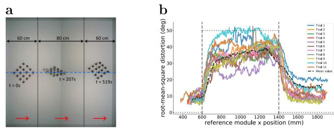
Fig. 4 | Physical experiments with  $4 \times 4$  Kilobot Soft Robots that are programmed to move forward, first in a square lattice shape, then in a compressed shape, and finally relaxing to restore their original shape. a Bird's-eye view of the experimental area, generated by superimposing snapshots taken from a typical experimental trial. The vertical dotted lines represent the positions where shrinking
