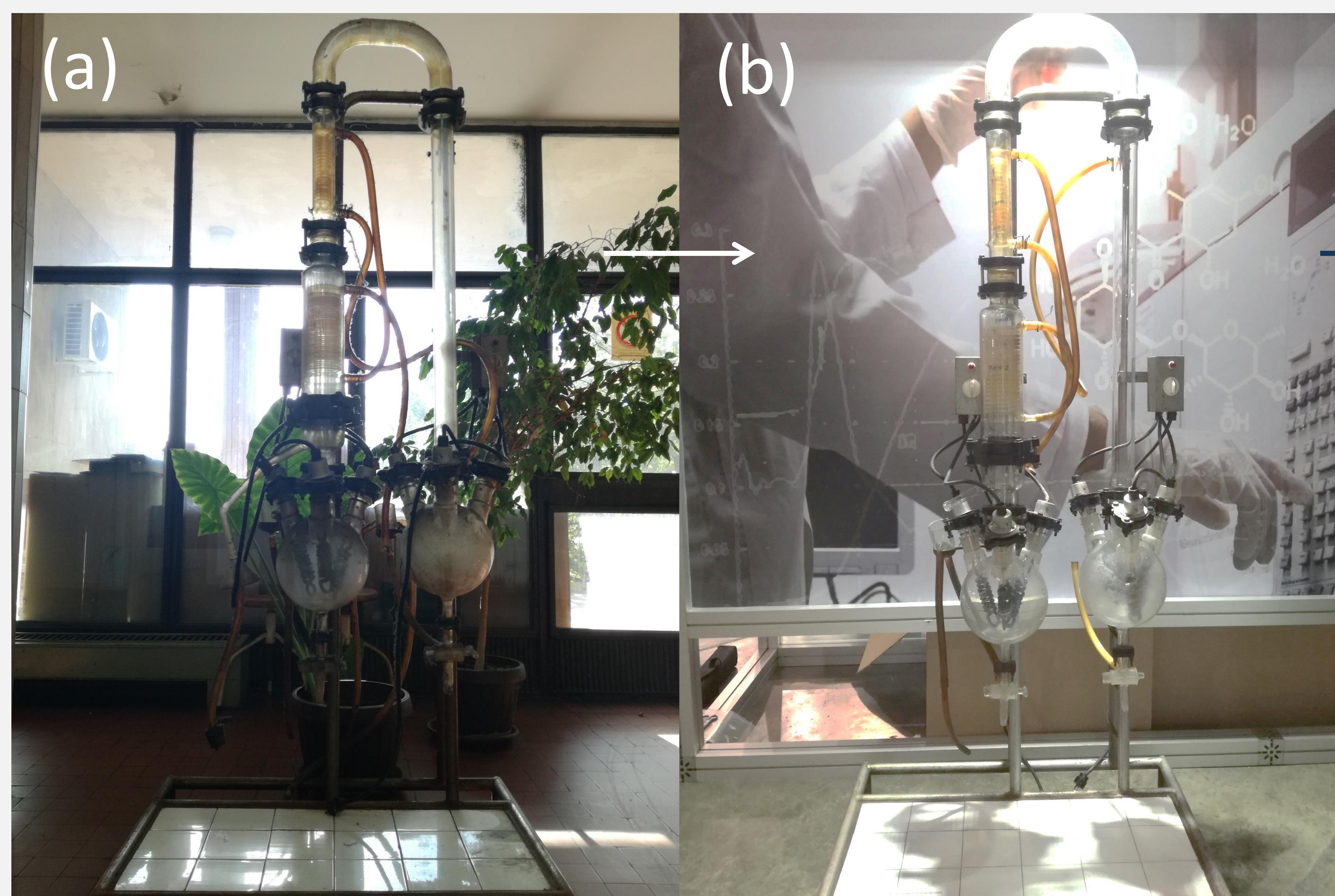
Fig 1. Apparatus for continual bidistillation of water, also known as Destilatron before (a) and after primary conservation (b)
