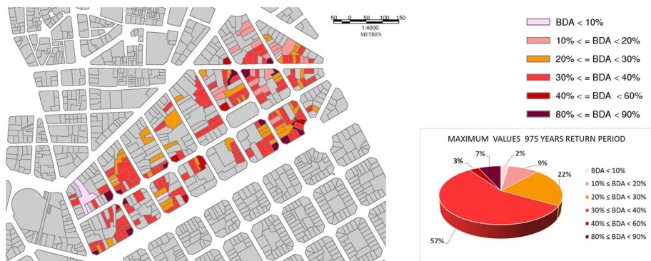
Fig. 32 Built damaged area. 975 years return period maximum values (in %). Façades 480 mm thick
