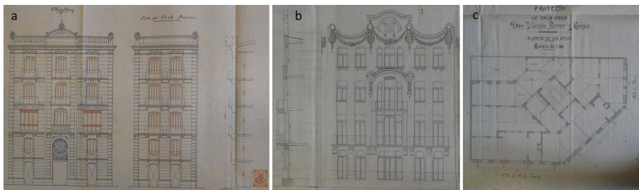
Fig. 12 Original building drawings. a facades and cross section. b facade and cross section. c building plan with load bearing walls. Source: Archivo Histórico Municipal de València. a AHMV Ensanche 1906 Caja 2 Exp nº 17 C/Cirilo Amorós 23. b and c AHMV Ensanche 1907 Caja 1 (26) Nº 94 EXP 12 H57 RG 4418)
