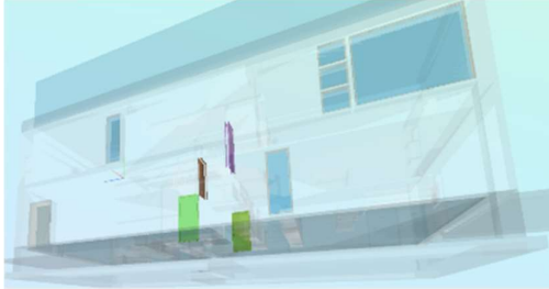
Figure 4: LD-BIM highlighting the four ‘non-compliant’ doors
