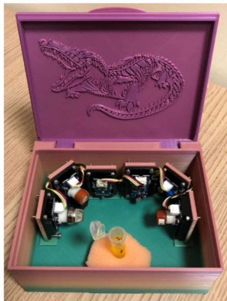
Figure 13. Photo of version 2 of the electronic nose used for the recording of different odours.
