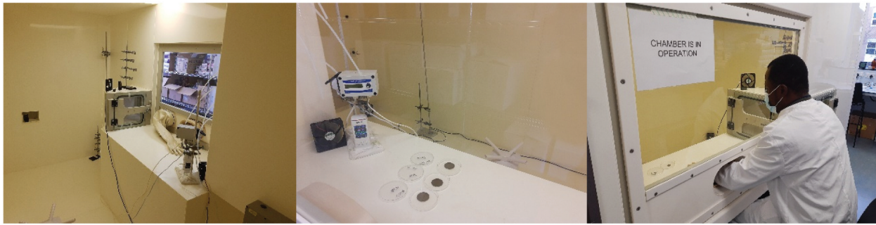
Figure 2. The internal and working area view of the bioaerosol chamber at Cardiff Metropolitan University. Left to right; Inside the chamber looking toward transfer port; Working area as seen from exterior showing steel discs in used in testing; the Author undertaking analysis in the working position.
