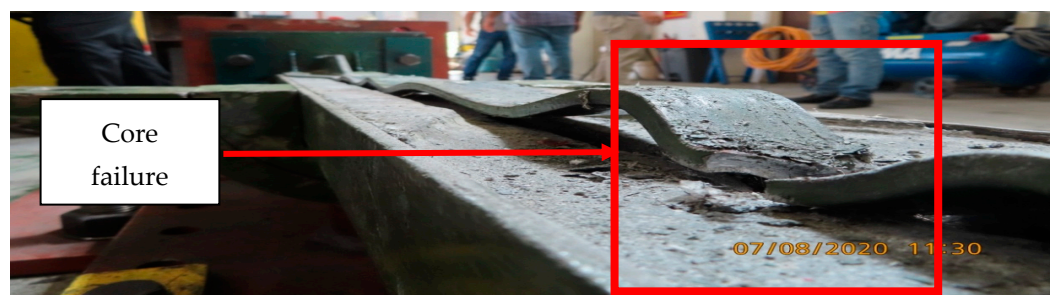
Figure 36. BRB core failure after testing.
