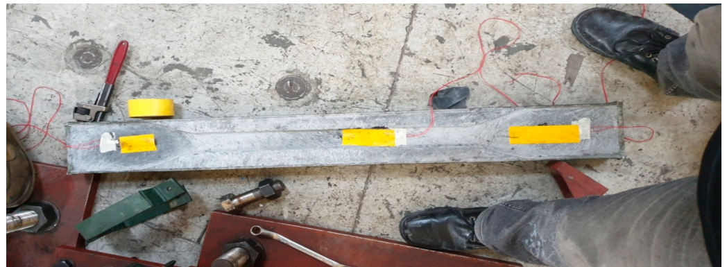
Figure 32. Location of strain gauges on concrete component.
