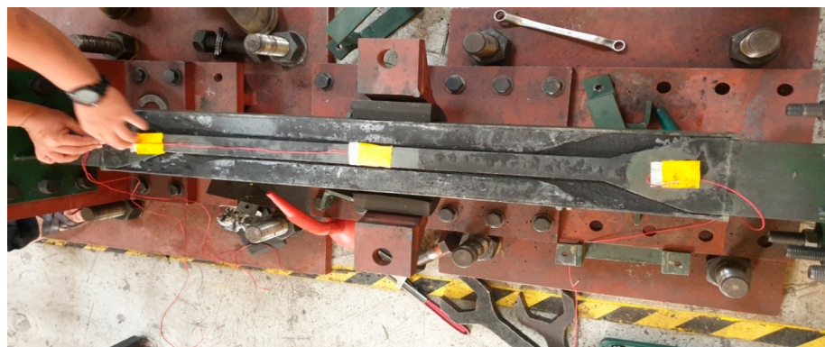
Figure 31. Location of strain gauges on steel core.
