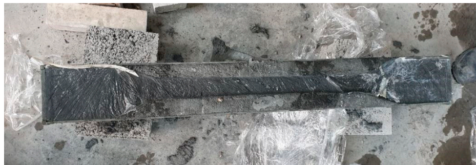
Figure 27. Cast concrete in BRB steel tube restrainer.
