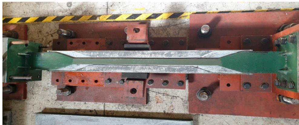
Figure 30. BRB installation in test setup.
