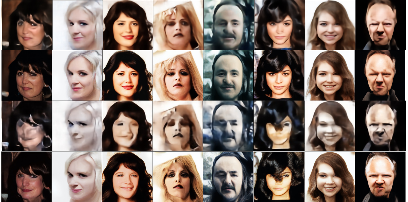
(b) First row: Reconstructions by DeepJSCC(CelebA-HQ), Second row: InverseJSCC(CelebA-HQ), Third row: DeepJSCC(ImageNet) and Fourth row: InverseJSCC(ImageNet), respectively, for SNR= 1.
