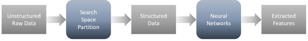
Figure 4.6: Illustration of the data post-processing pipeline. Unstructured raw data descriptive of a solution population P_g^r at generation g and run r in the form of tuples (\mathbf{x}, f(\mathbf{x})) of candidate solutions and fitness values are converted by a search space partitioning method into a structured data format \mathbf{z} , which subsequently can be fed to an adequate neural network architecture for feature extraction.
