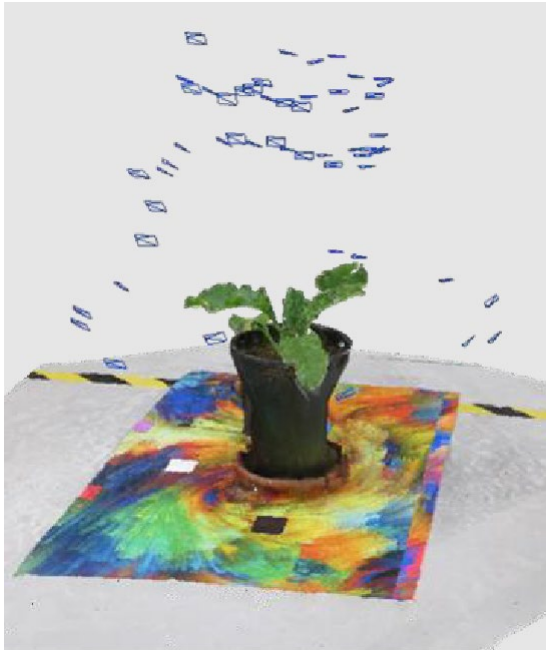
Figure 5.1 Camera positions from multi-view images. Each blue rectangle represents a point of image capture.
