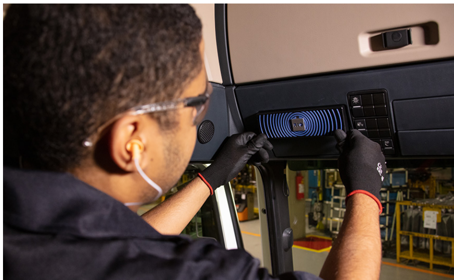
Figure 10. Assembly of Rio electronic module on VWCO plant
