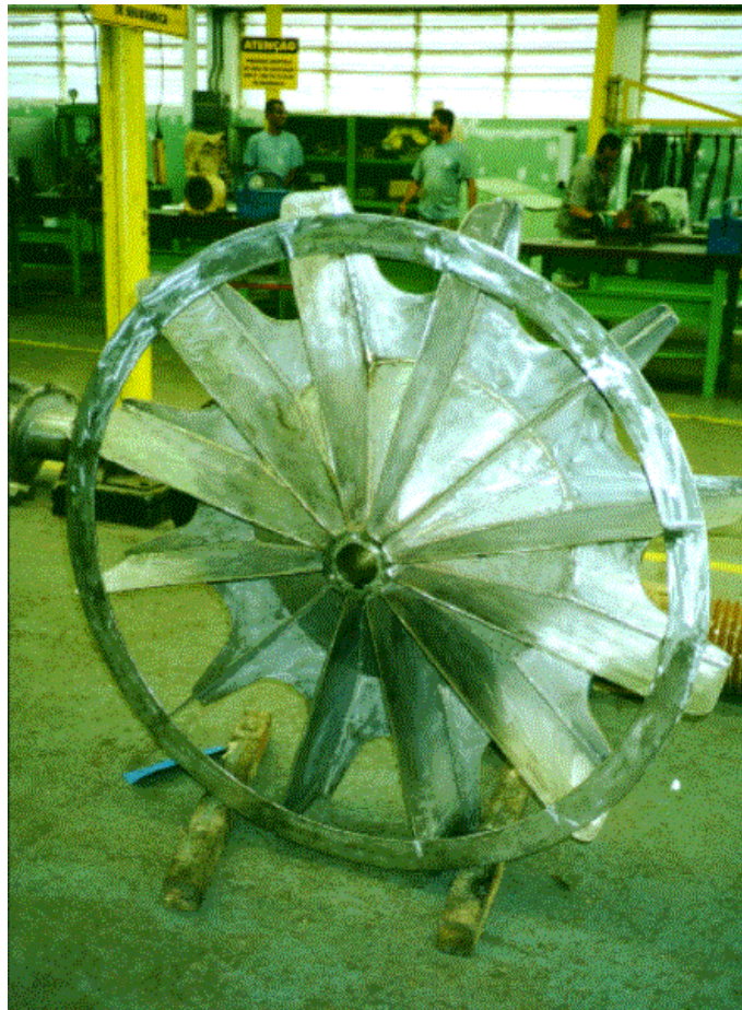
Figura13. Anel travando as pás do rotor
