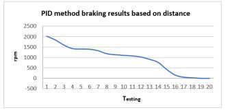
Fig. 23. Graph of PID method braking results based on distance
