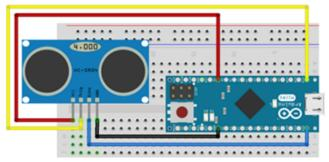
Fig. 9. HC-SR04 ultrasonic pin circuit
