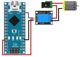
Fig. 11. DC motor pin circuit
