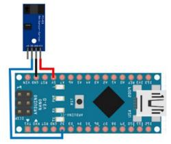
Fig. 10. Rotary encoder sensor pin circuit
