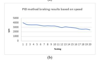
Fig. 28. (a) Results of braking without PID and (b) Results of braking with the PID method
