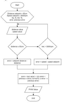
Fig. 14. PID control flowchart
