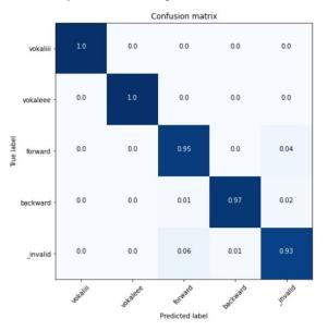
Fig. 15. The confusion matrix of testing model results. The y-axis represents the true label and the x-axis represents the predicted label for SCR classes
