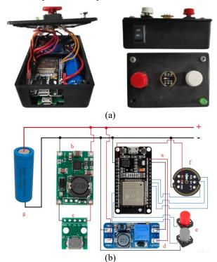
Fig. 8. (a) ESP32-master controller. (b) ESP32-master schematic
