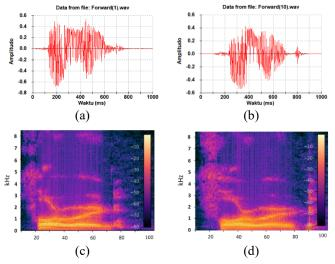
Fig. 10. (a) Time domain signal "Forward-1". (b) Time domain signal "Forward-2". (c) Spectrogram "Forward-1". (d) Spectrogram "Forward-2"
