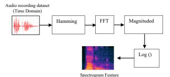
Fig. 4. The proposed STFT with 1x downsampling spectrogram for model features
