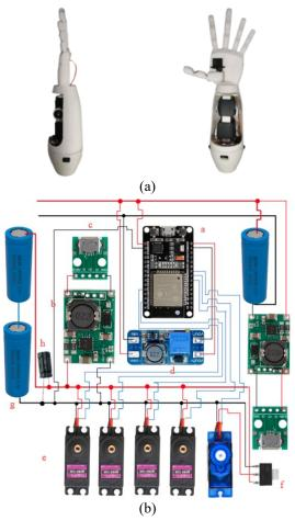
Fig. 9. (a) ESP32-slave prosthetic. (b) ESP32-slave schematic
