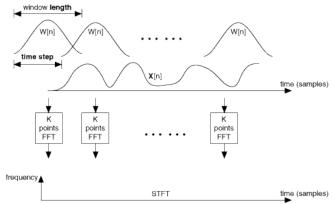
Fig. 3. Time domain voice signal transformation with STFT with hamming window
