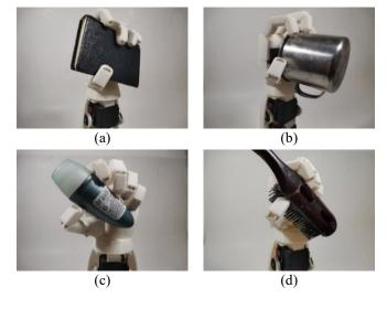
Fig. 16. Photographs ROM Activities, demonstrate Proto-1 grasping objects of various shapes. (a–d) Grasping a Qur'an, grasping a metal mug, grasping a deodorant, and grasping a comb
