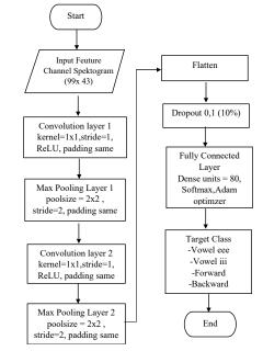
Fig. 6. Proposed flowchart 2DCNN architecture
