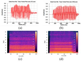
Fig. 11. (a) Time Domain Signal "vowel eee-1". (b) Time Domain Signal "vowel eee-2". (c) Spectrogram "vowel eee-1". (d) Spectrogram "vowel eee-2"
