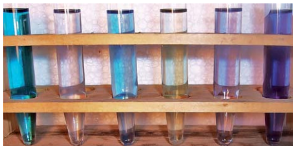
Fig. 2. Fractions collected during flash chromatography of a commercial lot of methylene green. The extreme left-hand sample corresponds to the purified methylene green; the extreme right-hand sample corresponds to methylene blue. The four center tubes correspond to unidentified impurities.
