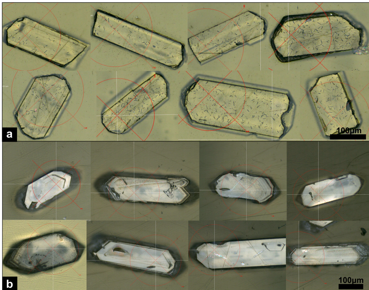
Fig. 8. Examples of the apatites (a) and zircon crystals (b) dated by fission track methodology. Zircon crystals describe uniform unaltered euhedral morphologies, and apatites euhedral to subhedral, both with well-developed crystalline forms and well-formed tetragonal prism faces. Photographs taken with Zeiss AXIO Imager Z2m binocular microscope, through TrackWorks Autoscan Software.
