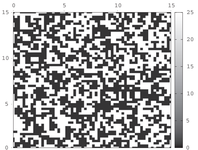
Fig. 9. Shear modulus of the fractal shale-limestone composite. Binary fractal of fractal dimension 2.2 and correlation length 0.06 in a scale of 10.
