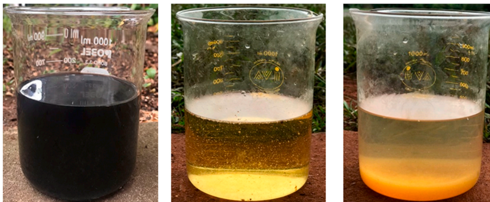
Fig. 5. Photographs of leachate samples before the Fenton process (left), after the Fenton process at pH 3 (center), and after neutralization at pH 6 (right).
