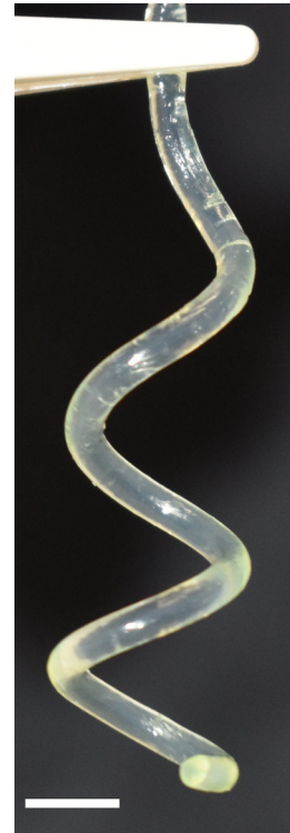
FIG. 5. Helix made of alginate (20 g/l) and agar-agar (10 g/l) suspended under its own weight. The white bar represents 5 mm.
