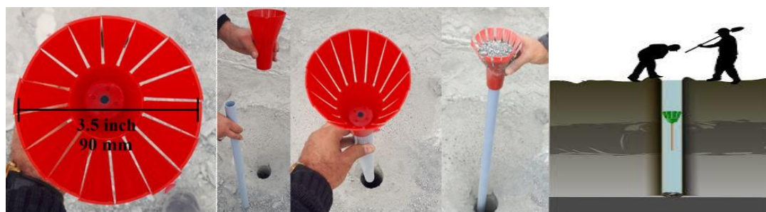
Figure 10. Assemblage of PVC pipe and basket.
