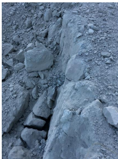
Figure 14. Separation of rock mass from stair wall and smooth wall in blast zone with air deck in Case 2.
