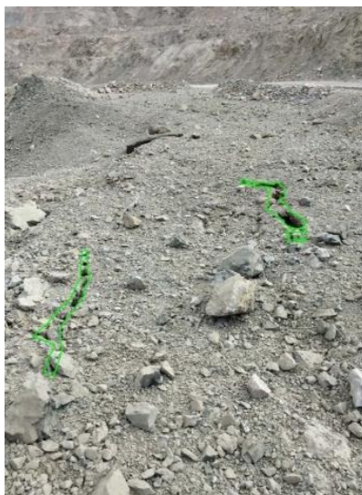
Figure 13. Back break in 3.5- and 4.5-in-diameter holes in the range without the air deck in Case 2.
