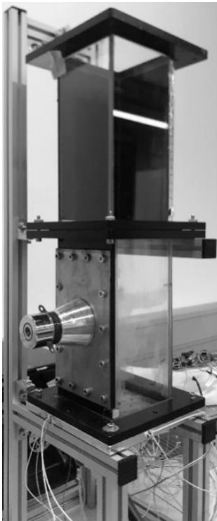
Figure 35. Lab-scale setup with ultrasound actuator clamped on metal wall
