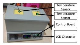
FIGURE 3. Digital Thermometer Calibrator Device Design
