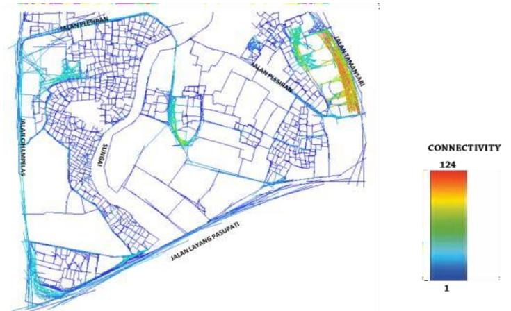
Fig. 3. The connectivity degree in the new scenario of potential street-network
