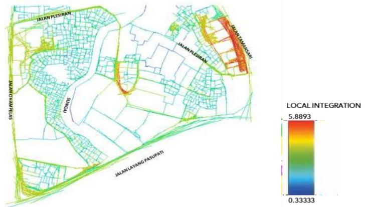
Fig. 7. The local integration degree in the new scenario of potential street-network
